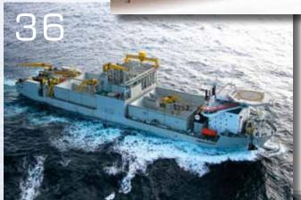
Front Cover: The 191m long Simon Stevin is deployed for accurate rock installations up to depths of 2,000 m. The vessel is in operation since late 2009 and has successfully completed challenging projects in Australia, Siberia and in the North Sea. Offshore Industry toured Jan De Nul's stone dumping vessel 'Simon Stevin' in the Port of Zeebruges, Belgium. More on page 36. (Photo courtesy of Jan De Nul/Imagen Naval 3kmi s.l.).
